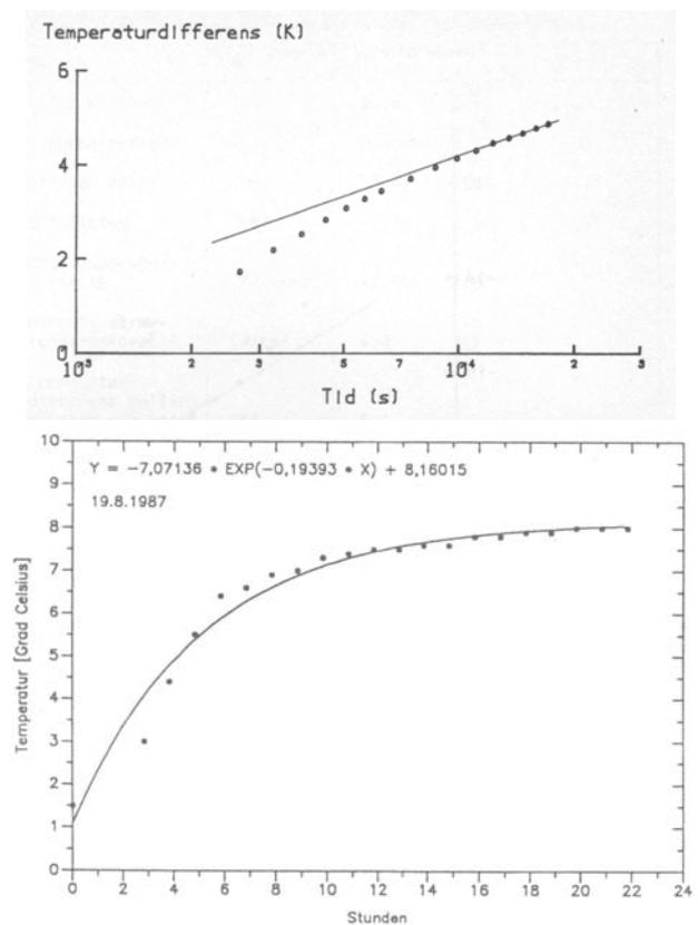
**Figure 3: Original graphs from temperature measurements for characterisation of BHE systems, development after stop of heat extraction; points measured and line calculated, on a logarithmic time axis (Mogensen 1985, top) and on a normal time axis (Knoblich et al. 1993, bottom)**
