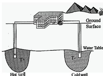
Figure 5: Schematic of an aquifer thermal energy storage (ATES)
