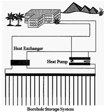
**Figure 3: Schematic of a borehole thermal energy storage (BTES)**
