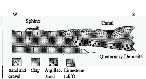
Figure 2: Geological cross section, showing contact of Quaternary aquifer with fractured limestone of the Pyramids plateau
