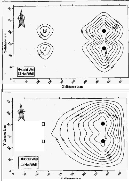
Figure 6: TRADIKON-3D simulation of one 250 kW ATES module with 2 + 2 wells (total of 4 modules for the building, i.e. 8 + 8 wells): Temperature distribution after 20 months (above) and after 9 years and 8 months (below); a volume of cold groundwater has accumulated around the cold wells.
