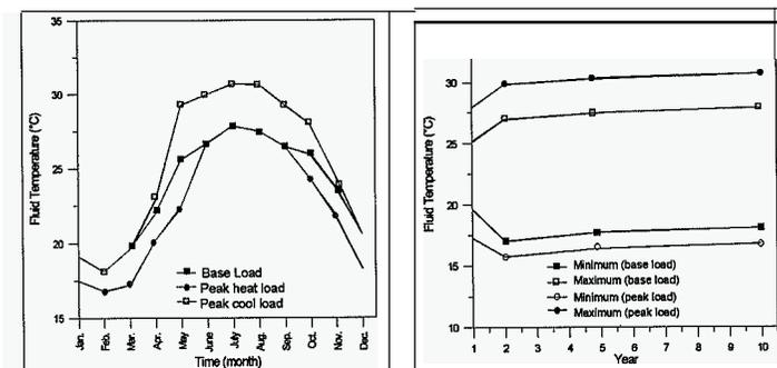
Figure 4: Fluid temperature development in the 10th year (left) and development of min. and max. fluid temperatures over 10 years (right), for BTES, calculated with EED
