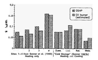
Figure 13: Cost of heating/cooling energy per kWh, incl. capital cost, in comparison to conventional design
