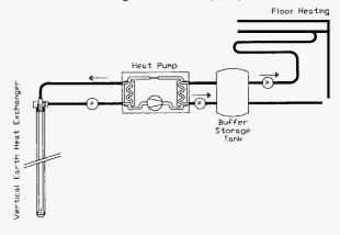
Figure 1: Schematic of "conventional" GSHP in Mid Europe
