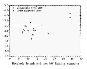
Figure 4: SPF versus layout parameter for exisiting GSHPplants with brine circuit resp. direct expansion.
