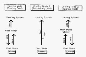
Fig. 9: Operation principles of GSHP-plants with cold storage
