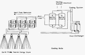
Figure 12: Schematic of "Technorama" Diisseldorf GSHP cold storage plant in 3 operation modes.
