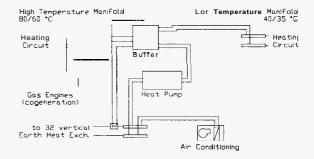
Figure 8: Schematic of GSHP-plant Frankfurt-Hiichst
