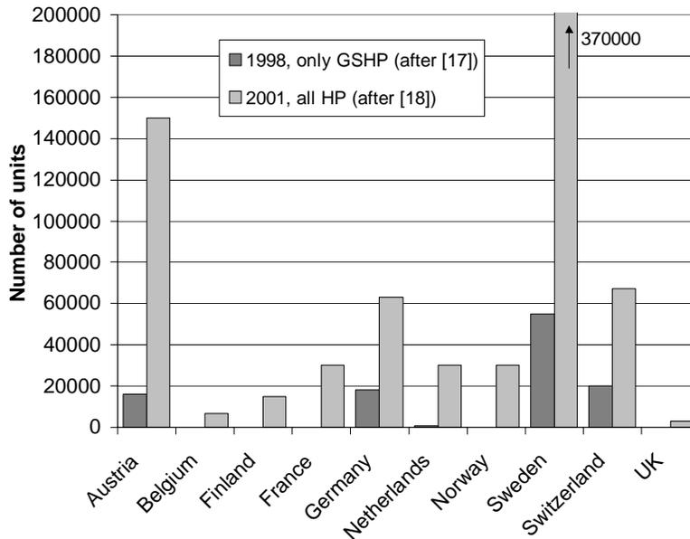
**Fig. 4: Number of installed heat pump units in some European countries (after data from Sanner, 1999; and Donnerbauer, 2003)**
